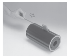
Clamp the setting block between head and clamping wedge to slide in the knife
