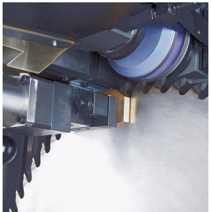
Machining of circular saw blades with outer diameters from 200 mm to 600 mm.
