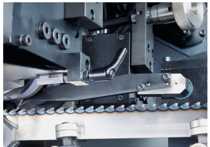
Fast-cycle feed system. Fast-cycle feed for narrow band saws, e.g. mini gang saw production (shortens the production time).
