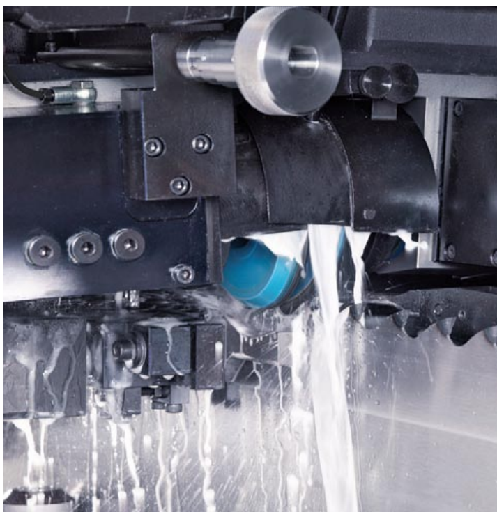
Grinding the tooth sides of band saw blades.
