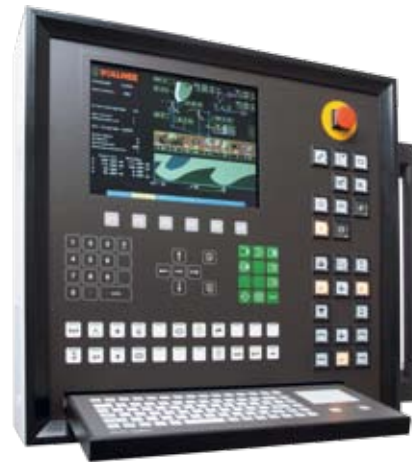
Control desk with input keyboard for program editing and data input
