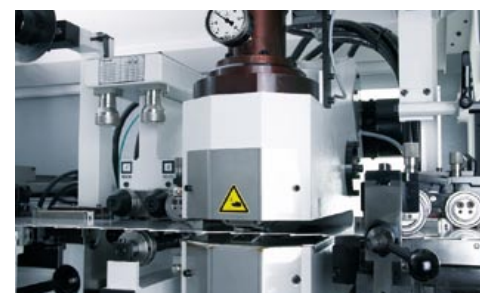
Tensioning and straightening station
